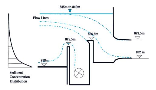
Scenario 2 – Sediment level at elevation 825.5 m asl
